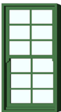
Sash and case window (Early 19th century) Lying pane style, common in Lanarkshire.
