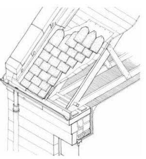
A junction between slating and stone skew can be formed with a mortar fillet or a lead flashing. But some movement should be allowed for in both cases
