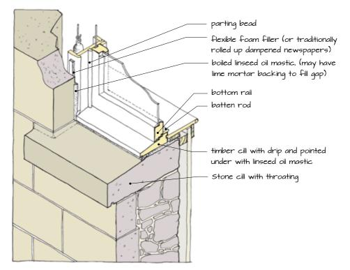
don't get painted and the cills and bottom rails take in moisture leading to decay. However such defects can also be repaired by experienced joiners at low cost.
