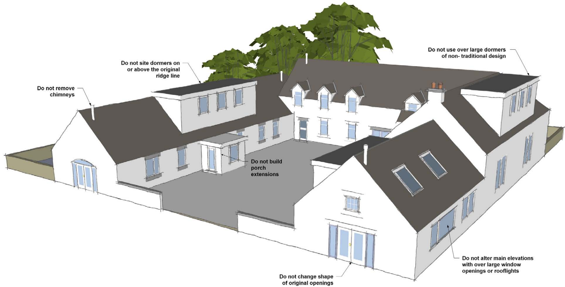
Figure 5.2 Poor example of the reuse of rural buildings
