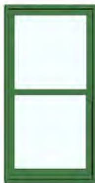
Sash and case window (Late 19th - early 20th century) Top sash may be smaller than lower sash.
