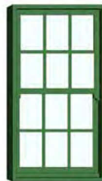
Sash and case window (1750 - 1830) 'Six over six' panes with strong vertical proportions. Earlier windows were smaller, with heavier frames of glazing bars.
