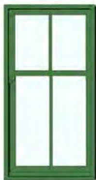
Sash and case window (Early 19th century) 'Two over two' panes with central glazing bar. Top sash may be smaller than lower sash.
