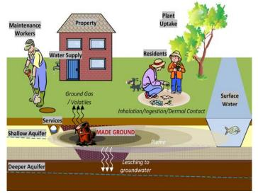
Conceptual site models are an essential element of the assessment and present the possible connections between identified potential contaminant sources, pathways and receptors.
